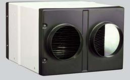
A ducted heat recovery unit for residential or commercial applications. The HR200V is self-contained and includes two mixed flow speed controllable fans. Using a high performance, polymeric heat exchange cube together with two power fans, the HR200V can boast a temperature efficiency of up to 70%. Low speed for trickle ventilation mode.
